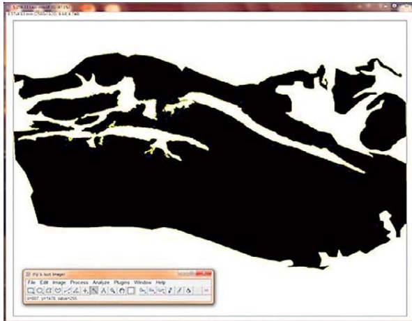
Fig. 3. Image shown in Figure 1 open in FIJI. The image was converted to 8-bit type image and thresholding was enabled for the wand tool, which was used to select the mask area, corresponding to the area of myocardial layer on the original image (yellow lining around the black mask denotes selection).
